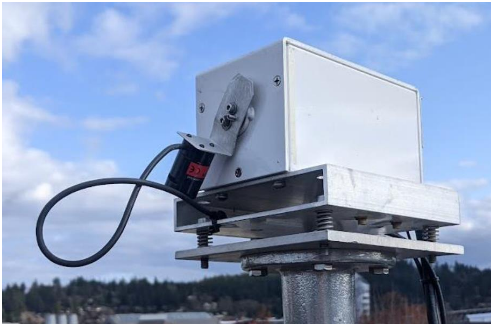
Figure 8: Head of the MPIS installed at SRML, sensor is at rest, waiting for the time to next sweep.
