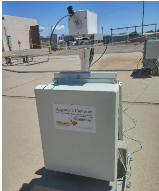
Figure 6: Multiplanar Irradiance Sensor (MPIS) by Augustyn & Company installed at PSEL. The sensor is in the middle of sweeping the pyranometer through its arc.
