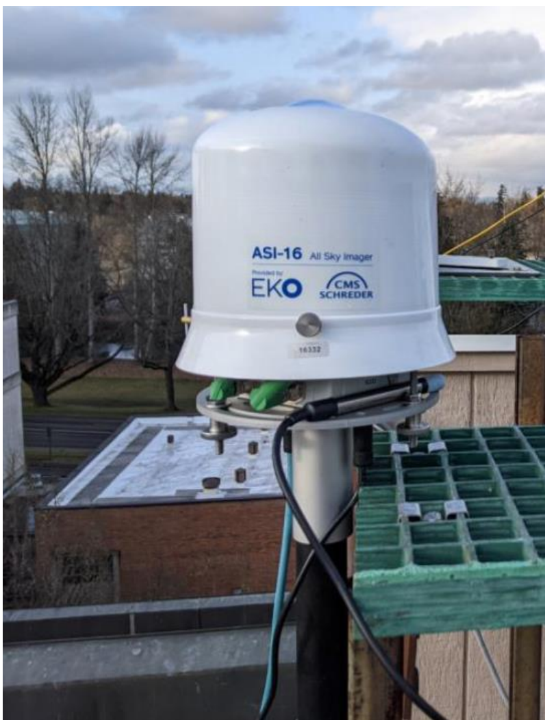
Figure 2: ASI-16 sky imager mounted at the SRML site in Eugene, OR.
