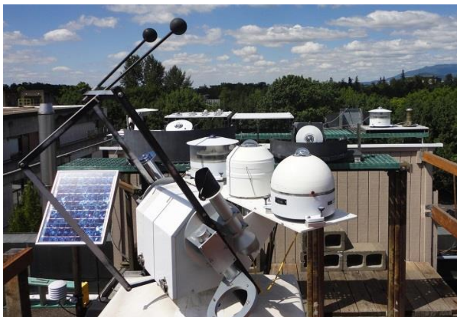
Figure 11: Irradiance tracker portion of the weather station at SRML
