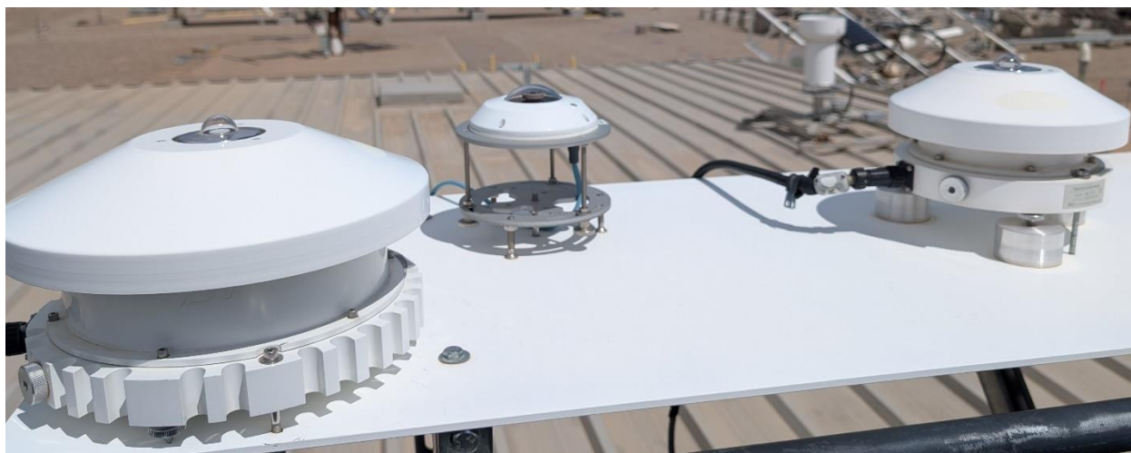
Figure 1: ASI-16 Basic sky imager (center instrument) between two other solar radiation measurement sensors at the PSEL in Albuquerque, NM. The instrument on the left appears in the sky images in the top right portion of each image.
