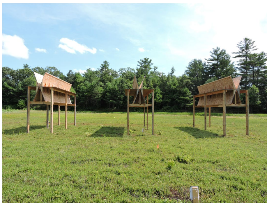
Figure 1. Prototype agrivoltaic system installed on a 'Stevens' cranberry bog at Carver, Massachusetts, USA.
